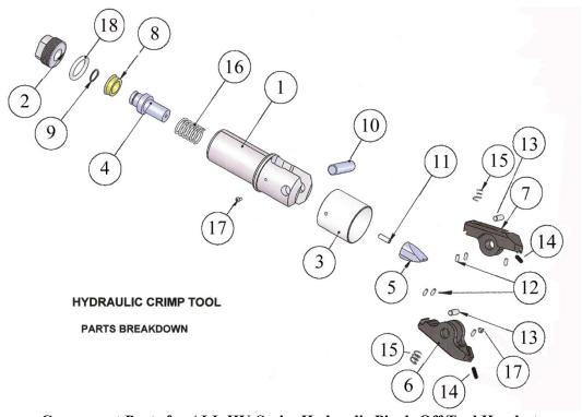
Component Parts for ALL HY-Series Hydraulic Pinch-Off Tool Handsets
